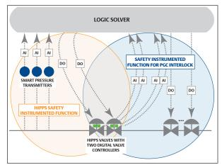
Updated architecture for HIPPS and PGC interlock with two digital valve controllers installed on each HIPPS valve.
