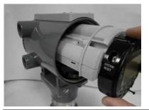
7. Connect the new battery to the open connector. Route the wires so they are in the recessed area. Make sure the wires don't get caught in the end cap threads.
