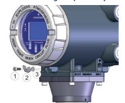
**Components of Retaining Clamp Assembly**
