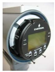
6. Grasp the HMI module and gently pull it and the battery pack out of the enclosure, leaving the battery still connected.
