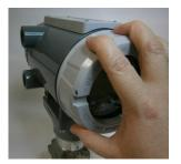
3. Unscrew the end cap turning it counter-clockwise until the cover comes off. Set it aside in a safe location.
