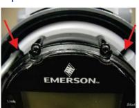
5. With a #1 Phillips-head screwdriver, loosen the two bottom captive fastening screws on the HMI module. Leave the two top screws on the HMI module connected to the battery pack.
