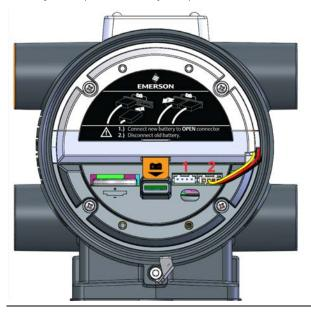
In the following procedure, you slide out the first battery pack (leaving it connected), attach the new battery to the second (available) connector (so both batteries are connected), and then disconnect the old battery pack.
