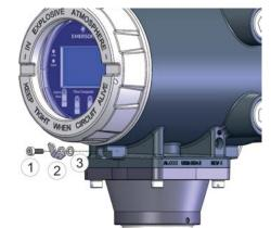
Components of Retaining Clamp Assembly
