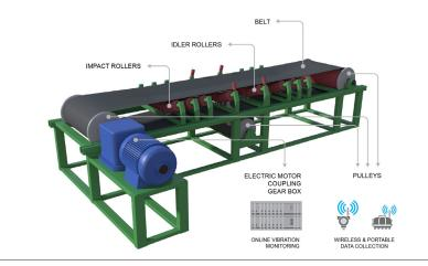
The ideal monitoring solution for a conveyor system includes a number of different sensing technologies.
