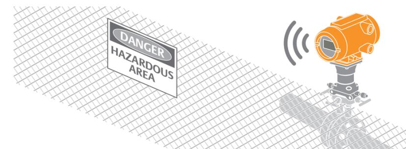
FBxWifi™ allows a secure local connection to the flow computer from a designated safe area for monitoring, data collection and configuration.
