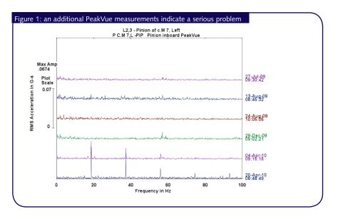
unusual. Then, additional PeakVue measurements made on April 20 revealed a big change. The five very apparent spikes in Figure 1 were the earliest indication of a serious problem. This is the story of using Emerson's PeakVue technology to make predictions of the bearing's expected run-life, which led to an order to stop the mill for repairs. In this case, the downtime was limited to about 12 hours to replace the faulty bearing.
