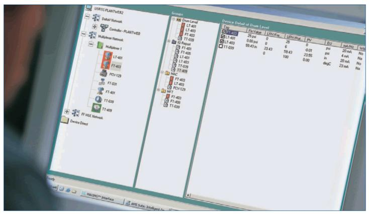
Interlock checkout is streamlined by grouping, monitoring, and fixing the output of HART transmitters from the convenience of an AMS device manager workstation.
