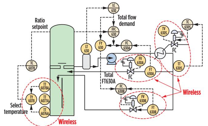
FIG. 4. Trapout tray level and liquid split control. Wireless temperature and flow transmitters are used.
