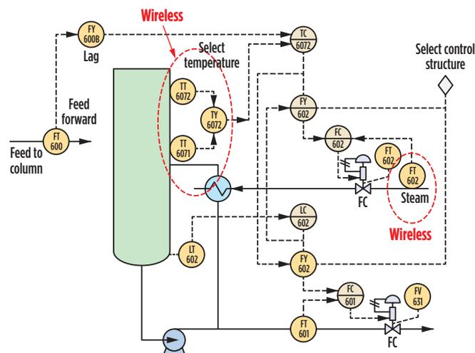
**FIG. 7.** MPC for DWC wireless temperature control.
