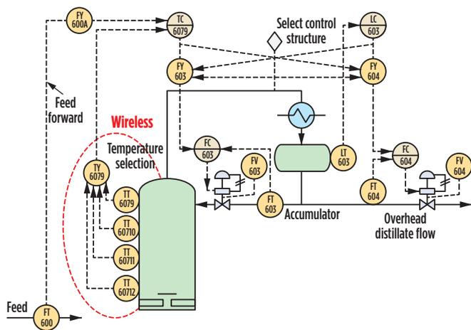
FIG. 3. Distillate and reflux flow control. The temperature transmitters are wireless.
