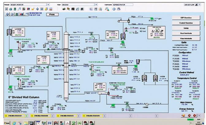
FIG. 10. Operator screen for DWC operation.
