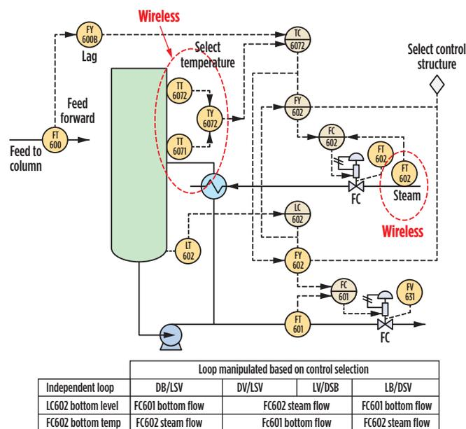
**FIG. 6.** Bottoms level and flow control.
