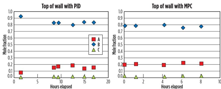
FIG. 13. Top of the wall mole fraction trends with PID and MPC control.
