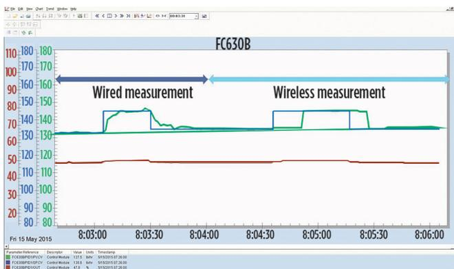
FIG. 8. Wired vs. wireless control of FC630B liquid flow.
