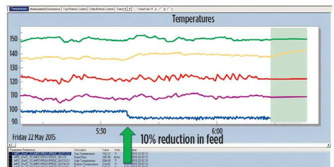
FIG. 11. Temperature trends for a 10% change in feed flow.
