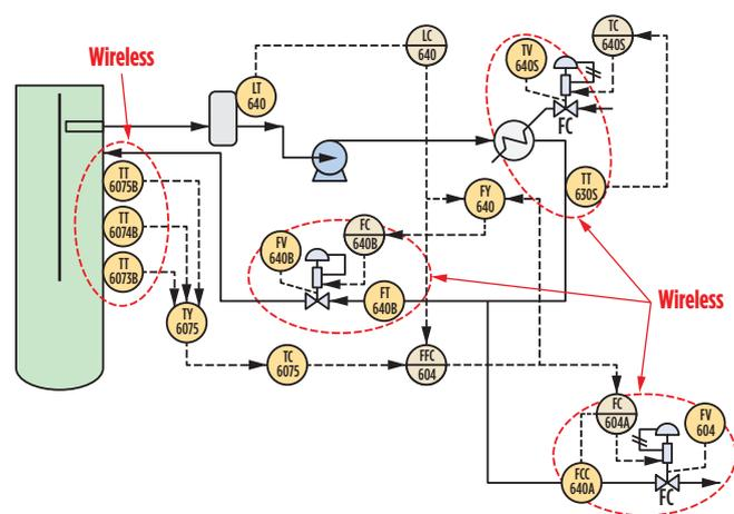
**FIG. 5.** Side-stream flow control.
