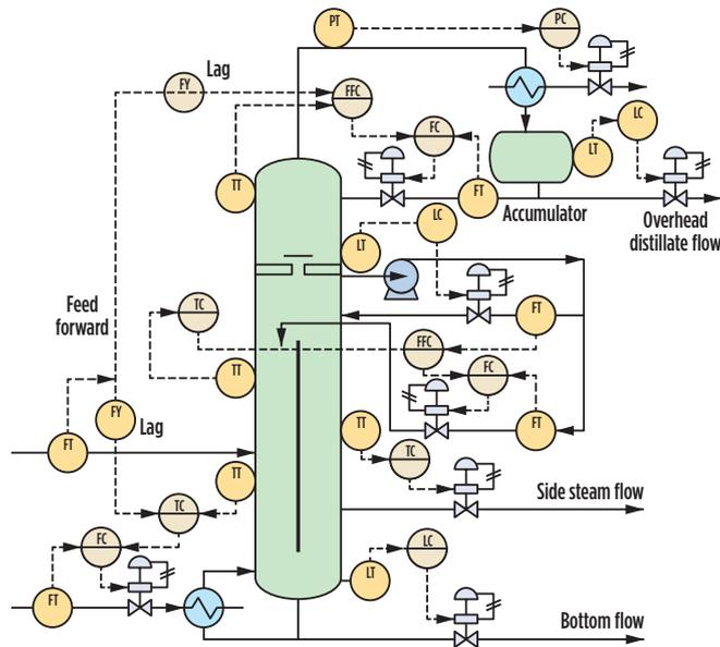
FIG. 2. Basic DWC control scheme, as proposed by Ling and Luyben in 2010.
