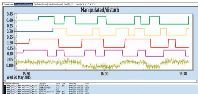
FIG. 9. The process test shown here developed the MPC model used for the University of Texas DWC.
