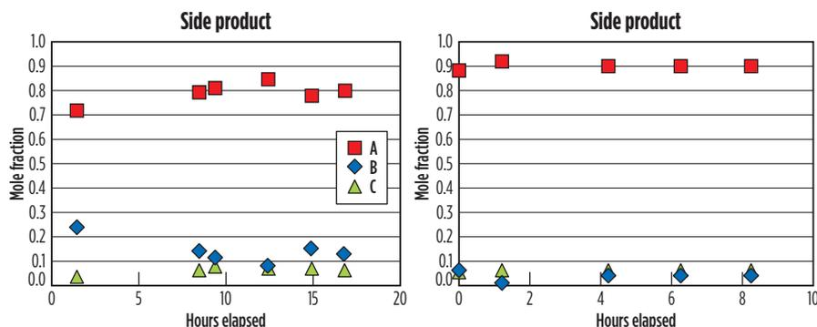
FIG. 12. Side-product mole fraction trends with PID and MPC control. With MPC, side fraction variability is significantly smaller than with PID.
