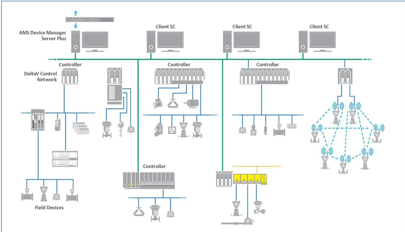
Using AMS Device Manager with the DeltaV system enables you to access important HART, FOUNDATION Fieldbus, WirelessHART, PROFIBUS PA, and PROFIBUS DP device data with no additional cabling or field wiring required!
