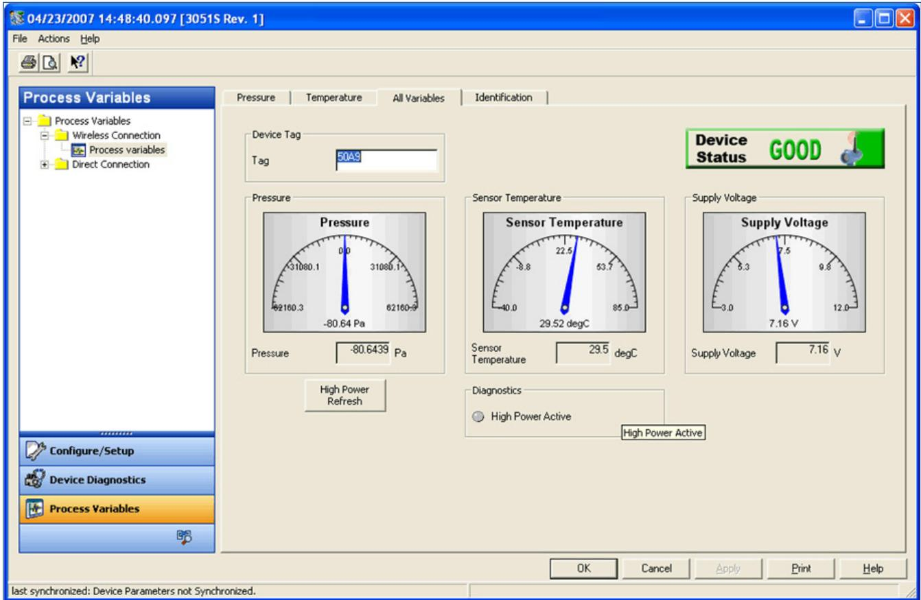
AMS Device Manager's enhanced graphical interface provides clear indications of device status and process variables, extending the benefits of Plantweb to WirelessHART devices.
