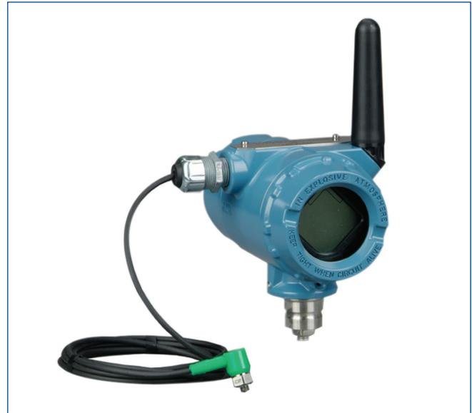
*The AMS 9420 delivers complete vibration information, including high resolution spectra and waveform, over a self-organizing wireless network for use by operations and maintenance personnel.*
