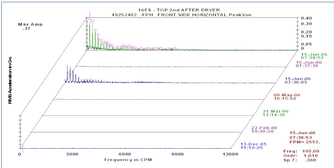
Because of production requirements, the bearing was flooded with oil to maintain TM operation. Readings on June 19, 2006 found that the audible noise and PeakVue values decreased. The problem still exists but was masked by excessive bearing oil. Recommendations to inspect the bearing and perform monitoring until maintenance was possible were reiterated.
