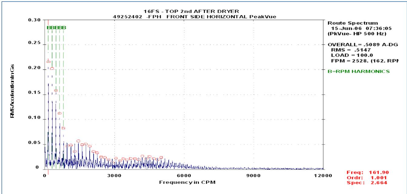
Three PeakVue readings were collected at that time, which are displayed in the waterfall plot below. The middle June 15th reading was taken when the audible noise decreased. An analysis of the collected data was performed and a report generated. Recommendations were made to increase monitoring of the bearing PeakVue and temperature values until maintenance could be performed. An inspection of the bearing for looseness or wear was also recommended at the next opportunity.
