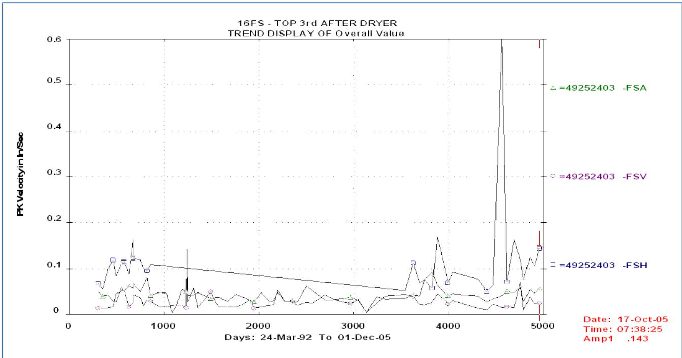
On June 15, 2006, vibration analysis was requested on the 16TM T2 After-dryer tending-side bearing. This was on the same After-dryer section of the tissue machine as the previous failure. An intermittent audible noise was emanating from the F/S T2 bearing. Vibration data was collected on the bearing along with PeakVue readings. Horizontal, vertical and axial vibration amplitudes were low, below 0.12 ips on the bearing housing readings.
