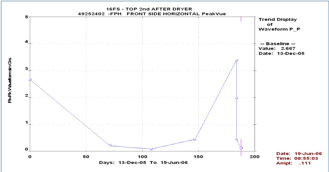
A TM shutdown was scheduled for June 20th and an inspection of the After-dryer T2 Roll bearing was performed at that time. The inner race was found to be loose on the shaft. Measurements on the journal found it to be severely worn where the bearing inner race was spinning on the shaft. A compression fit is used on this configuration to hold the inner race in-place on the roll journal. The journal was machined and a sleeve was installed along with a new bearing.
