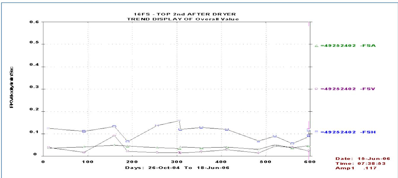
PeakVue data contained multiples of TS, and the overall PeakVue value increased when the audible noise was louder.
