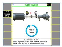
Sweep laser heads. Start anywhere. Stop anywhere. Minimum recommended sweep size is 45°. Press [ENTER] to retrieve data via Bluetooth.
