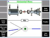
When viewing the Horizontal Move screen, press [F12] for 'LIVE MOVE'. Place laser fixtures in desired position and press [ENTER] to start.
