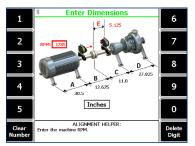
Optional machines types enable entry of values for C and D for the other machine. Note: Use [./] to calculate fractions. Example: 30 3/8 = [3] [0] [./] [3] [./] [./] [8]
