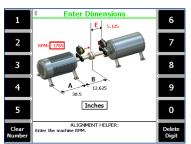
Values for A, B, E and RPM are required. Use [<] and [>] to move between fields.
