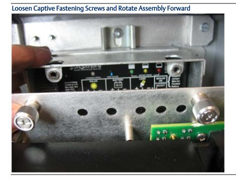
4. If you have an internal solar regulator installed in the battery compartment, you must remove the termination cover. Remove the two screws (left and right) that fasten the termination cover to the solar regulator, and then set the termination cover aside. (If you don't have an internal solar regulator, skip to Step 5.)
