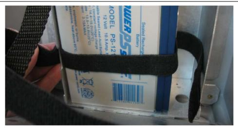
12. The strap includes a narrow opening into which you can slide the other end of the strap to help you tighten it.
