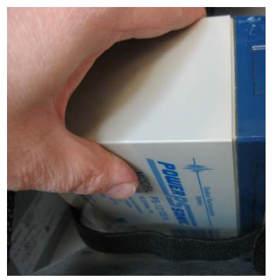
11. Carefully push the battery under the solar regulator (if present) and against the back of the compartment, now strap it in tightly by pulling the ends of the strap.
