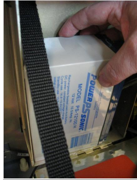
Pry Out Old Battery Pack (Leaving Connected to Cable)
