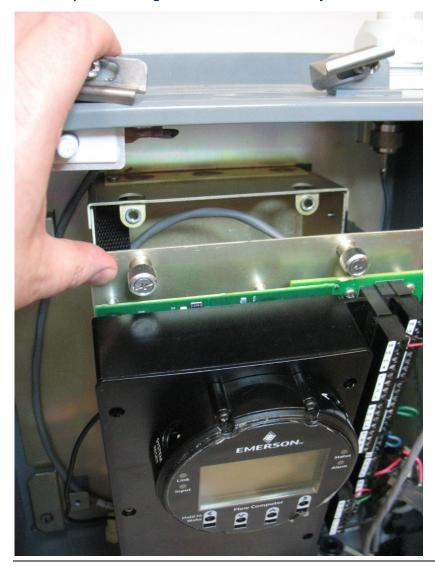
4. A VELCRO brand fastener on the back of the battery secures it to the back of the battery compartment. Leave the connectors on the current battery connected. Place your fingers behind the battery pack and pry it off of the fastener on the back of the compartment; you may need to use both hands. Gently lift the battery with the battery cable attached out of the compartment. You may want to place it on top of the flow computer enclosure.
