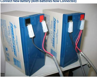
Connect New Battery (Both Batteries Now Connected)
