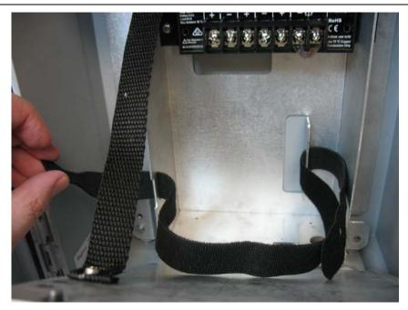
10. Pick up the new battery and carefully ease it into the battery compartment with the writing on the battery facing out and the connectors on the upper right-hand side. Nothing (including the strap) can be **behind** the battery.
