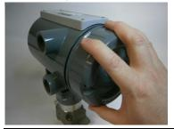
3. Unscrew the end cap turning it counterclockwise until the cover comes off. Set it aside in a safe location.
