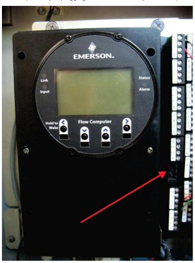
3. Disconnect the intermediate cable between the CPU enclosure and the sensor module. To do this, press down on the outer edge of the connection tab, then pull the connectors apart.
