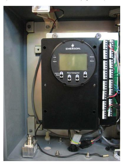
2. Remove power by unplugging terminal block TB2 (pins 1,3,5,7).
