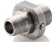
**WARNING: To prevent the possibility of death, personal injury, or property damage, the two Slip-Lok connectors halves must be fully seated together and both locking screws tightened to 20 in. lbs. [2,3 Nm]. Ensure that the Slip-Lok connector is secure before placing into service.**
