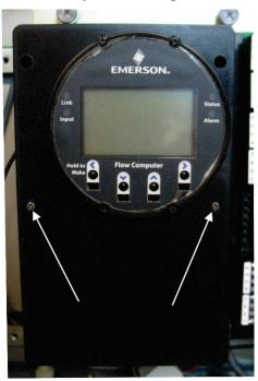
Removing the CPU Enclosure Cover
