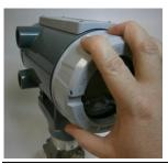
3. Unscrew the end cap by turning it counter-clockwise until it comes off. Set the end cap aside in a safe location.
