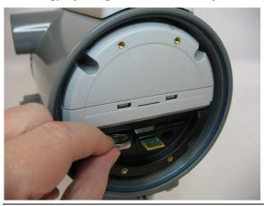
7. Insert the new coin cell battery in the slot. The positive side (+) must be on top.
