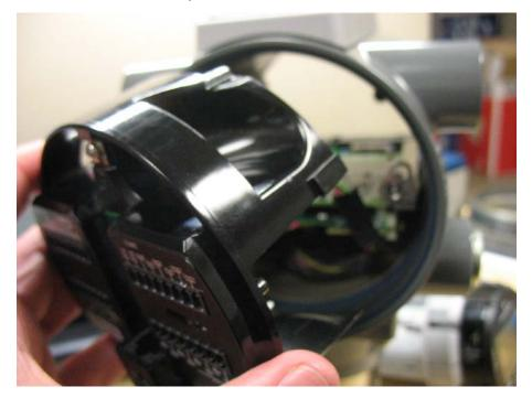
14. With a #2 Phillips-head screwdriver, loosen the two captive fastening screws in the plastic bezel that hold the CPU module in place. (To preserve data, **do not** remove the SRAM backup battery.)
