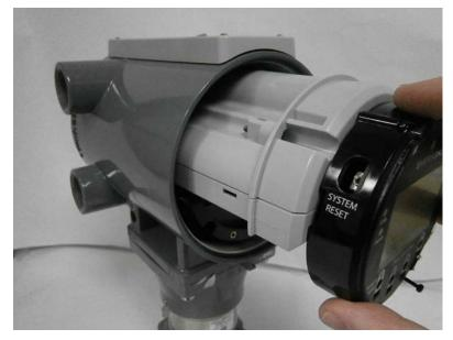
9. If the battery pack enclosure holds an internal battery, disconnect the battery connector.
