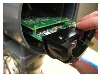
16. Use a 3/32-inch flathead screwdriver to separate the internal wire connector plug from the plug on the bottom of the CPU module.
