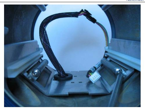
18. Looking into the **front end** of the enclosure, pull the card cage out of the enclosure, then disconnect the upper part of the sensor cable and push the lower part through the grommet so you can completely remove the card cage. Set the upper part of the sensor cable aside; you will need it later.
