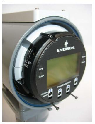
8. Grasp the HMI module and gently pull it and the battery pack enclosure out of the housing.
