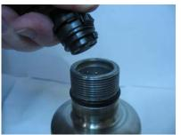
22. Press the sensor cable onto the connector of the new (replacement) sensor assembly.
