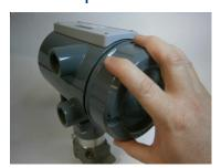
3. Unscrew the end cap turning it counter-clockwise until the cover comes off. Set it aside in a safe location.
