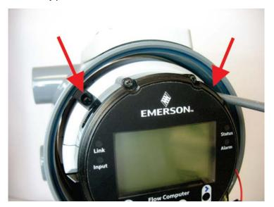
7. With a #1 Phillips-head screwdriver, loosen the two bottom captive fastening screws on the HMI module. Leave the two top screws on the HMI module connected to the battery pack enclosure.
