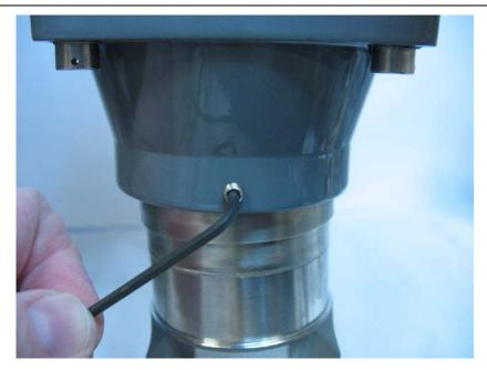
20. Grasp the sensor with one hand and unscrew the flow computer housing with your other hand until you can lift it off. Then set the enclosure aside.
