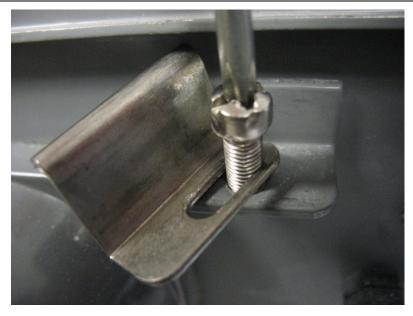
2. Place the new clamp in place so it holds the lip of the door. Tighten the screw to hold the clamp in place. Torque screw to 18 to 20 in lbs (2 to 2.3 N m).
