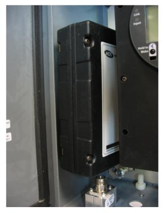
3. Use a #2 Phillips-head screwdriver to loosen the two captive fastening screws on the radio bracket above and below the radio.
