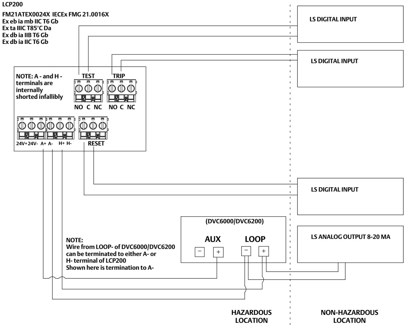
Figure 7. Explosion-proof, External Power 24V, ATEX/IECEX
