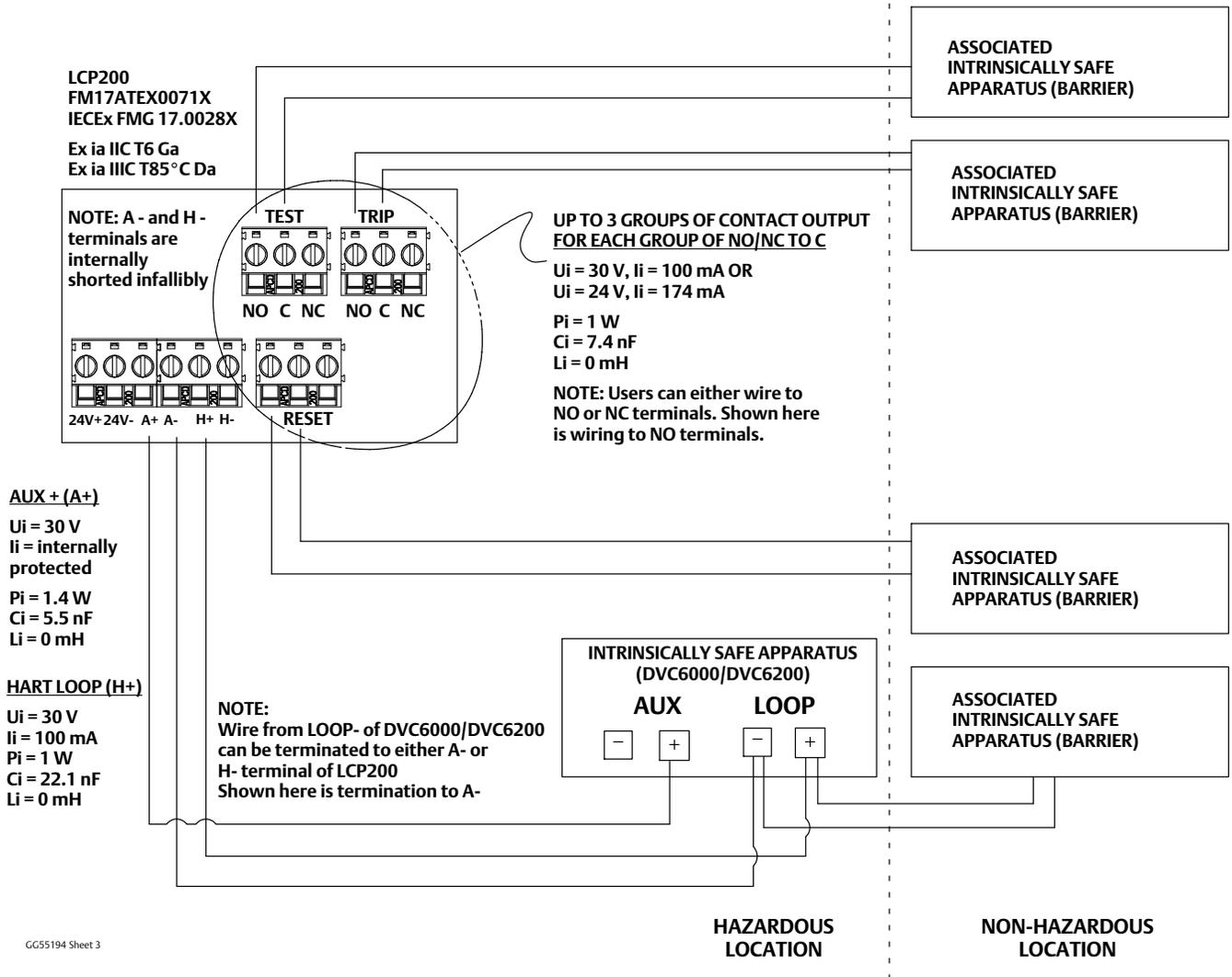
Figure 2. Intrinsically Safe, External Power 24V, ATEX/IECEX
