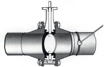
2. Tack weld the flanges to the pipes.
