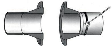
3. Remove the valve and finish weld. Install the valve according to the procedure in the left column.
