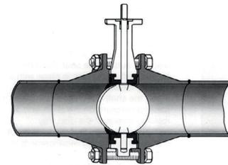
2. Open the valve and remove the flange spreads.
