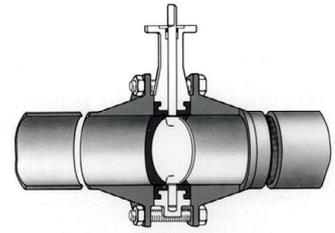
1. Center a flange-valve-flange assembly between the pipes.
