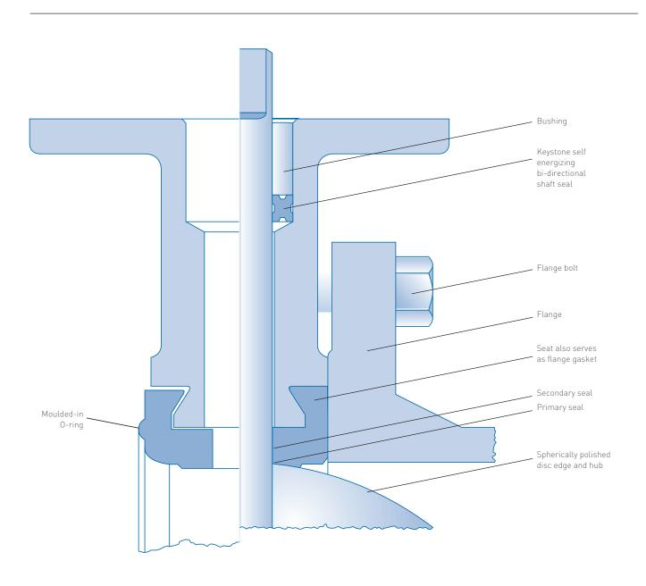
Resilient seal systems for F129, F139, F990, F239 and F2000 series butterfly valves
