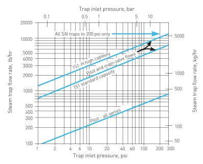
Note: 151-H High Capacity Trap - use 1" pipe, valves and fittings.
