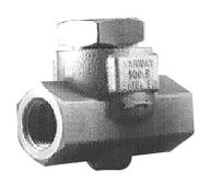
The Series 151 Dual Range Steam Trap is designed for use on both batch and continuous applications such as batch stills, autoclaves, reboilers, storage tanks, shell and tube heat exchangers and tank coils. The Dual Range Steam Traps are capable of handling high startup and running loads, and provide maximum air venting capability.
