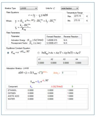
The Kinetics Guide provides knowledge and instructions on how to define the reaction type, reaction order, and evaluate the reaction parameters from the available experimental data. It provides a more detailed insight into the reaction kinetics, including the reactor types, general models for each type of the reactors, and basic definitions and relations of the chemical kinetics.
