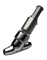
Emerson uses third party technology for a modulating solenoid valve, in response to the plant's flow control command. This technology consists of a pilot-operated solenoid valve, a LVDT for position indication, and a proprietary electronic positioner to create a closed feedback loop. It is particularly well suited where a pneumatic supply, required for traditional control valves, cannot be provided.
