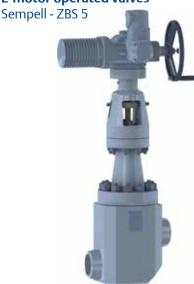
Bellows-sealed, Z-form forged body, high quality material, cobalt free hard facing at seat, disc and guiding surfaces. Different control characteristics available, permanent flow over throttle in the valve disc to keep the spray lines and the volume compensation line at a given temperature.
