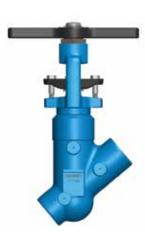
T or Y pattern bellows sealed globe valves designed for applications where process fluid leakage to the environment is unacceptable, e.g. radioactive, toxic, combustible, liquid metals, vacuum and helium gas, etc.
