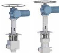
Electric-motor operated Gate and Globe valves for severe accident mode, capable to open at parameters up to 600 °C with a deltaP of up to 190 bars and able to stay open with pressurizer gas temperature up to 1200 °C. In addition, the valves are operable in the feed and bleed conditions.
