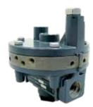
This pneumatic booster is used in conjunction with a positioner on a throttling control valve to increase the stroking speed.
