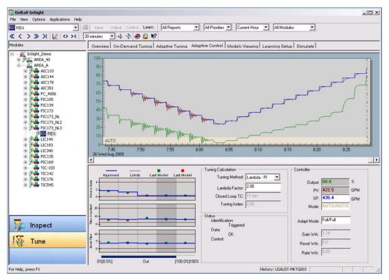
DeltaV<sup>™</sup> Adapt provides continuous adaptive control for any DeltaV PID control loop.
