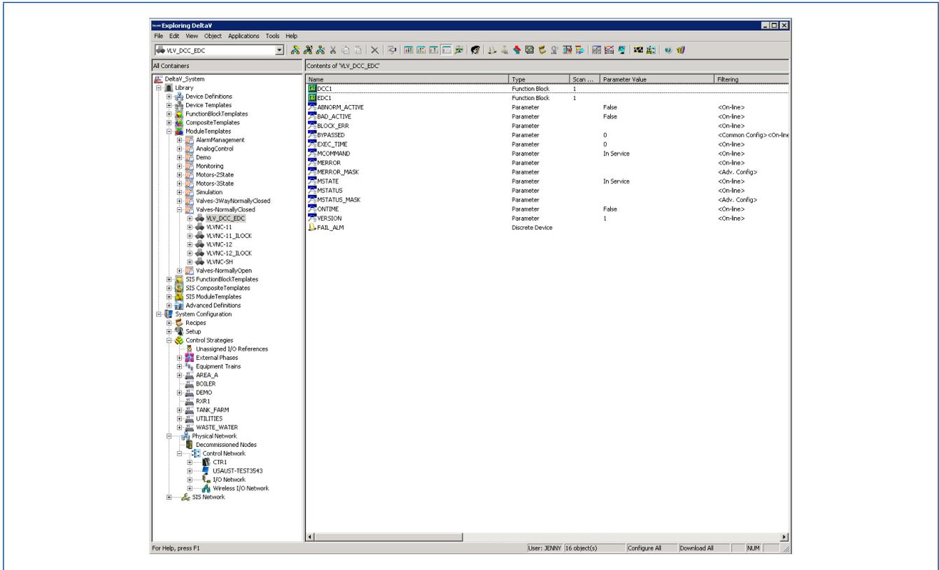
The DeltaV Explorer centralizes all system configuration tasks, including alarm, control and smart device configuration.
