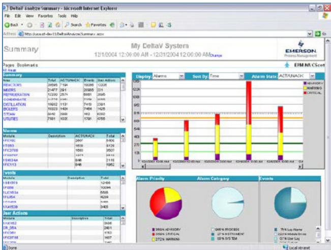
Quickly detect alarm patterns with DeltaV Analyze.
