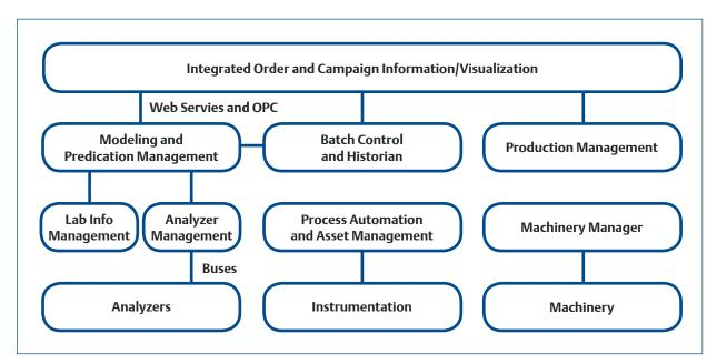
**Figure 1** — Emerson Integrated PAT Architecture: It is important to note that this architecture supports the capability for the customer to select the analyzers and modeling packages that best fit their particular PAT requirements.
