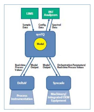
In this example, both DeltaV and Syncade are being used as data sources to the input blocks of a synTQ orchestration and the synTQ orchestration is integrated into a Syncade recipe work instruction.
