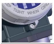
To loosen or tighten the screw, use a 3mm hexagonal wrench. When tightening, torque to 12 in-lbs (1.4 N m).
