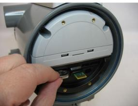
5. Insert the new coin cell battery in the slot. The positive side (+) must be on top.
