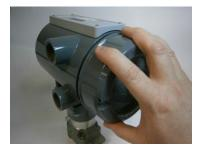
3. Unscrew the end cap turning it counter-clockwise until it comes off. Set it aside in a safe location.
