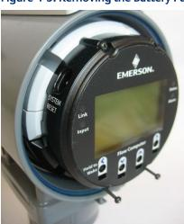
Figure 4-5: Removing the Battery Pack
