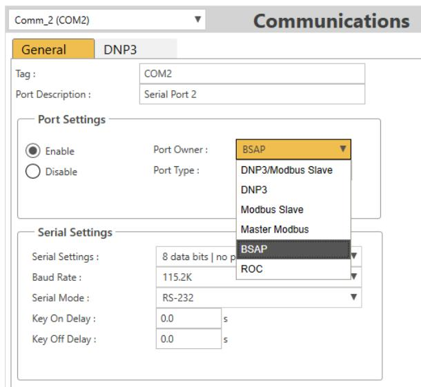
4. Modify the **Serial Settings**, **Baud Rate**, and **Serial Mode**, if needed, otherwise use the defaults shown in FBxConnect. Click **Save** when complete.
