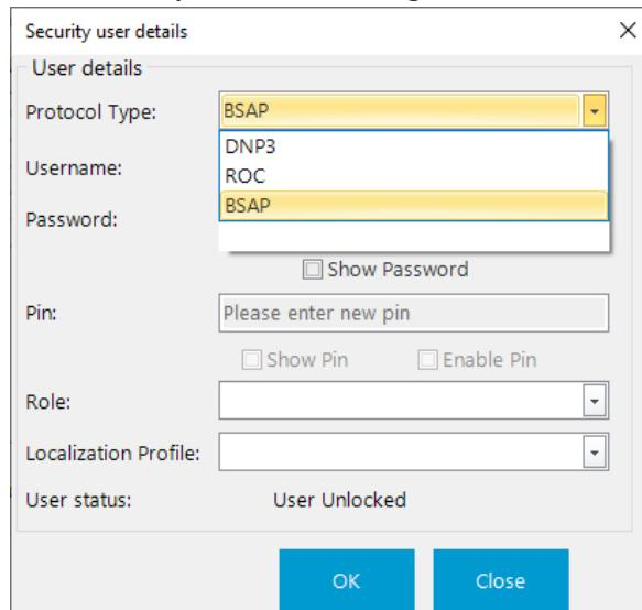
4. Create a user with a **Username** of **SYSTEM** and with a **Password** that matches the password for your OpenEnterprise SYSTEM user. (If you are not using OpenEnterprise, you could use a different username and password combination.) The Role for the SYSTEM user must be Admin or Engineer.
