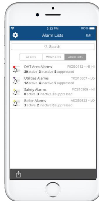
**Figure 6.** Example of a DeltaV Mobile Alarm List.
