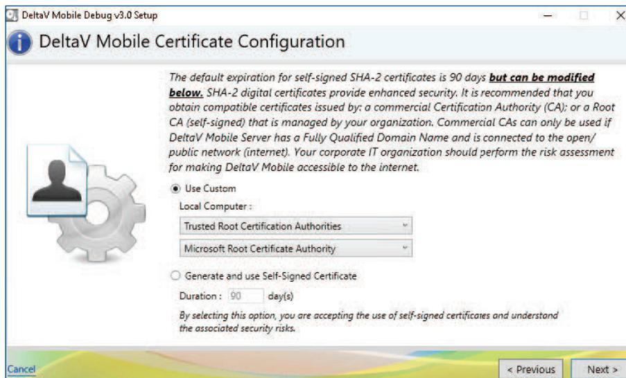
**Figure 9.** During installation of DeltaV Mobile, it can be configured to use certificates installed on the server.
