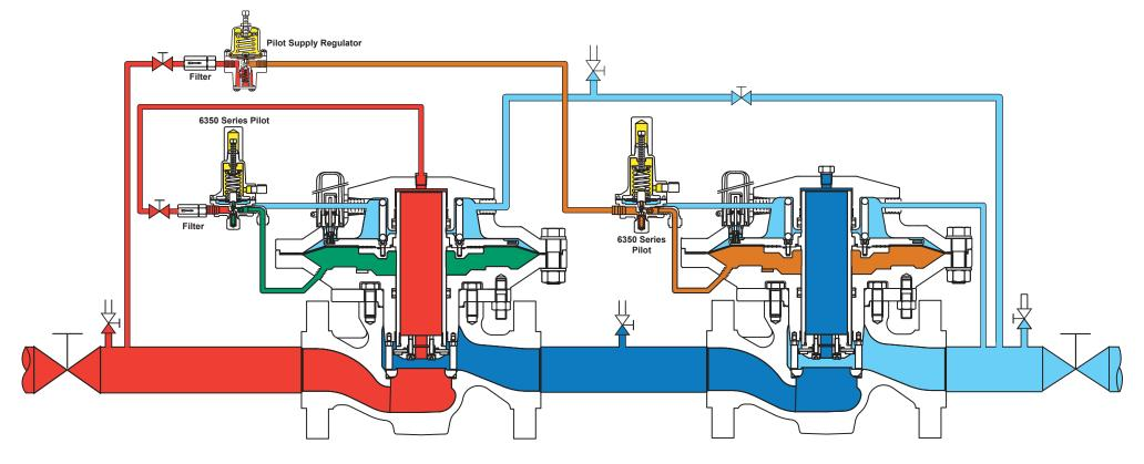
INLET PRESSURE OUTLET PRESSURE ATMOSPHERIC PRESSURE LOADING PRESSURE INTERMEDIATE PRESSURE PILOT SUPPLY PRESSURE
