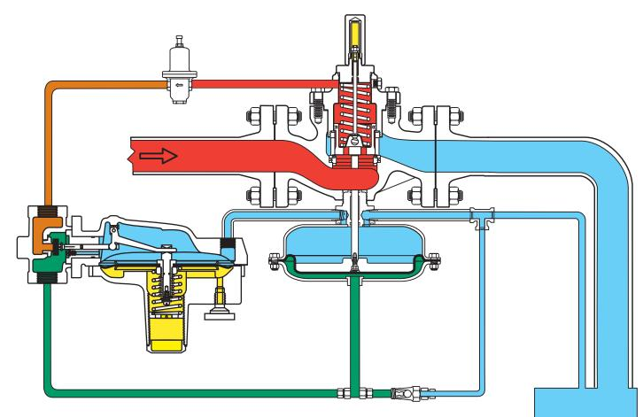
INLET PRESSURE OUTLET PRESSURE ATMOSPHERIC PRESSURE LOADING PRESSURE PILOT SUPPLY PRESSURE
