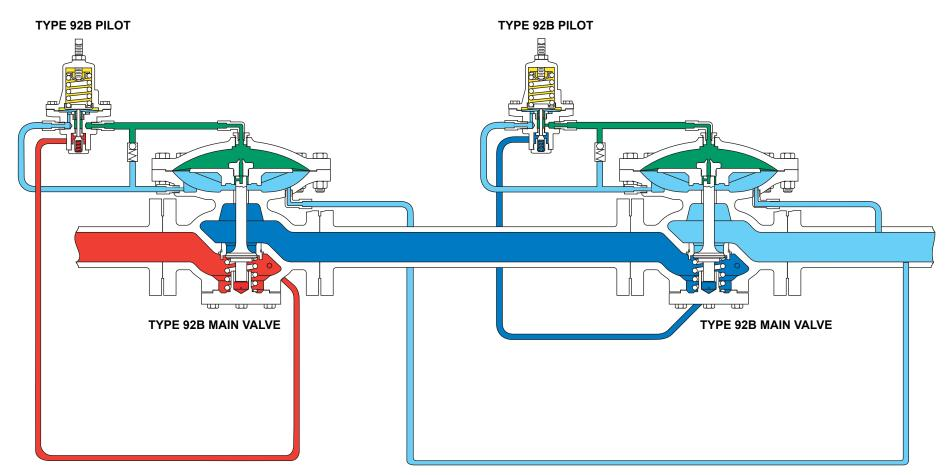
INLET PRESSURE OUTLET PRESSURE ATMOSPHERIC PRESSURE LOADING PRESSURE
