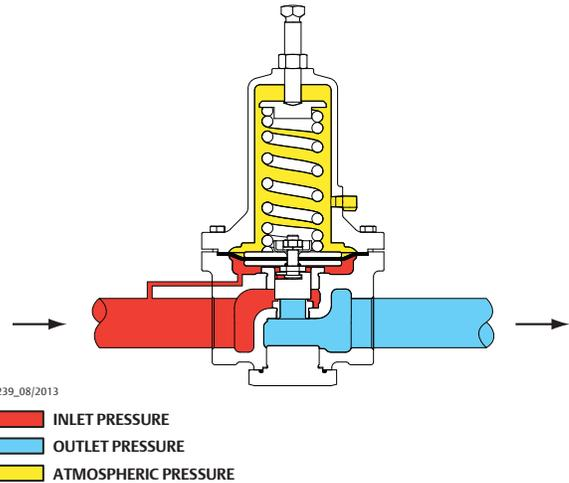
Figure 2. Backpressure Regulator Operational Schematic
