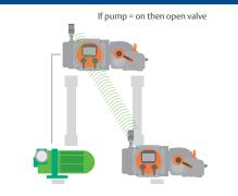
**Prevent untimely operation** with a built- in inhibitor interlock system that prevents operation with other devices until external contact has been made. Your systems can now coordinate with each other.
