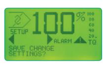
Your displays need to show the right information without being too simple or complex. Easy to read IconoText displays and icons allow for an easy and intuitive setup. If overtorque = true then stop all functions
