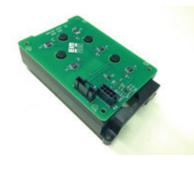
Absolute Position Detector provides precise valve position under all conditions including loss of power, no battery backup required.
