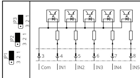
**Figure 83. 2 Separated Groups of 2 Inputs with Same Ground Input IN3 is Disabled**
