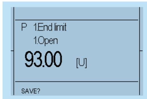
Step 9 - In order to confirm the end position (save), slightly flip up the selector switch towards ☑ and let it snap back to its neutral position.
