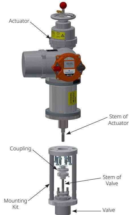
**5.2.2 Alternative Procedure for Valve with Required Sealing Force**
