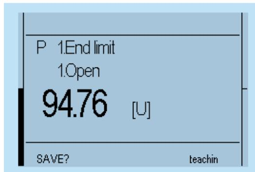
Step 7 - Manually move the actuator with the handwheel (see Section 3.5) or by motor via the control switch (black button) to the end position OPEN of the valve.
