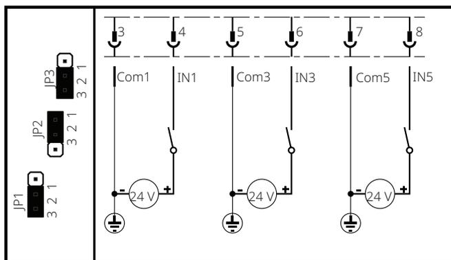
**Figure 90. 3 separated Inputs with Common = "+" Using External 24 V**
