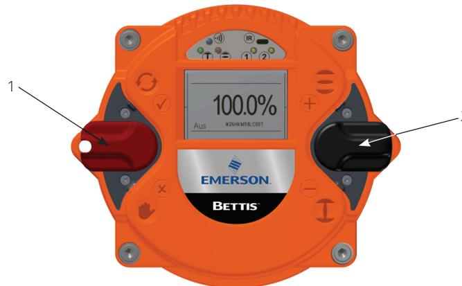
Step 2 - Now, move the control switch down (towards) until the menu item "P20.6 Miscellaneous - Wireless" is displayed.
