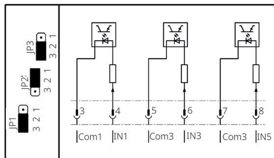
**Figure 85. 3 Inputs with Same Common and 1 Separated Input IN4 is Disabled**
