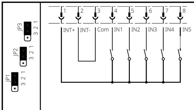
**Figure 89. 3 Separated Inputs Using 3 Separated External 24 V**
