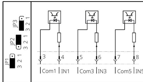
**Figure 86. 1 Separated Input and 3 Inputs with Same Common Input IN2 is Disabled**
