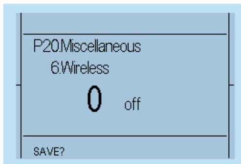
Step 5 - Flip up the control switch (towards) to change the value from 0 (off) to 2 (Bluetooth).
