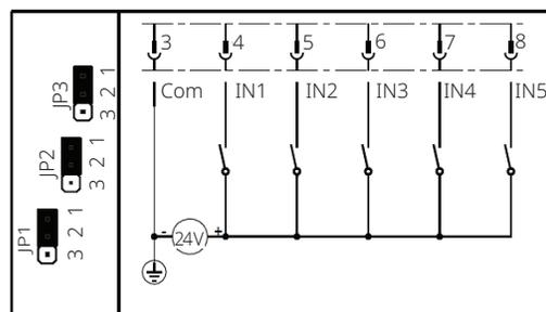
**Figure 88. 5 Inputs with Common = "-" Using Internal 24 V (e.g., for dry contacts)**
