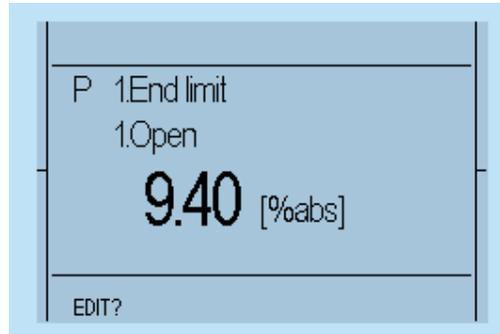
During operation, the display shows the position of the actuator as a percentage, operation mode and status. When using the option "identification", a customer-specific label is shown at the bottom of the display (e.g., PPS Number).
