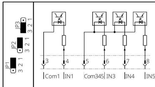
**Figure 87. 5 inputs with Common = "-" Using External 24 V**
