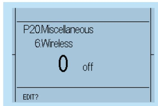
Confirm the selector switch (with a slight flip upwards, towards ↕, (see Figure 26 to Figure 30) to change the selected parameter. To confirm this input readiness, the display changes from "EDIT" to "SAVE".
