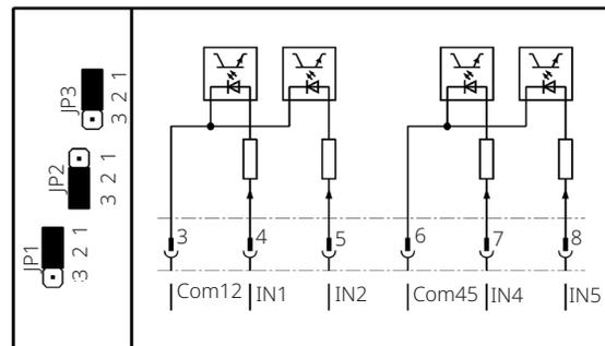
**Figure 84. 3 Separated Inputs; Inputs IN2 and IN4 are Disabled**
