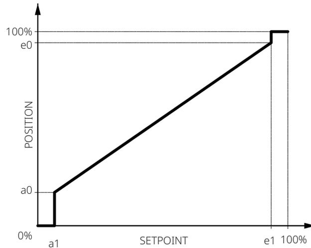
**Figure 62. Function Principle of the Deadband, and Hysteresis in Conjunction with the Positioner**
