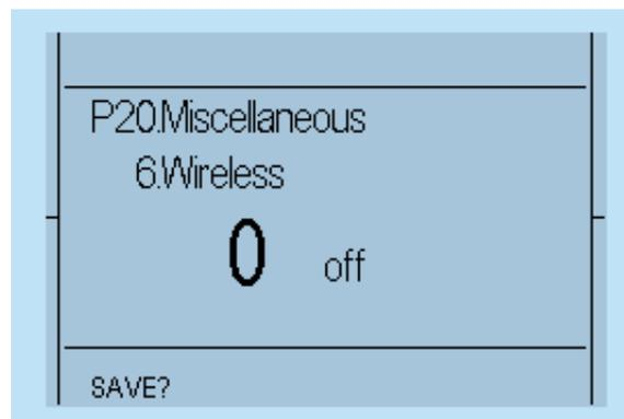
Move the control switch towards to the characters to change the parameter. ⊕ or ⊖ (see Figures 37 to 40). After reaching the desired parameter value, confirm the value with the selector switch (again, flip it slightly towards ✓, (see Figures 26 to 28).
