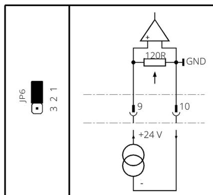
**Figure 92. Input with Internal Supply (Active Input)**
