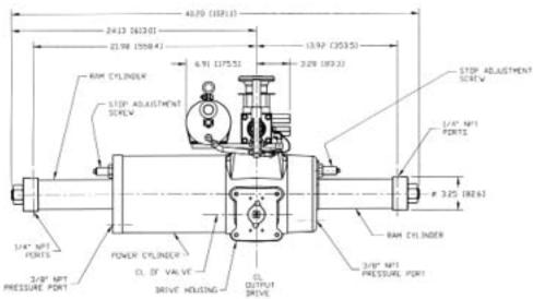
ACTUATORS SHOWN ROTATED TO FULL CLOCKVISE POSITION
