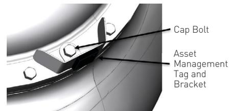
FIGURE 3 - 90/9000 SERIES PILOT-OPERATED VALVE CONFIGURATION WITH ASSET MANAGEMENT TAG
