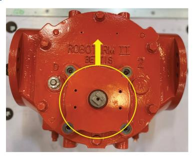
**2.1.3** Remove the position indicator assembly (1 - 140) from the actuator.
