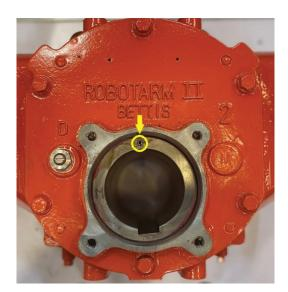
**2.2.2** Pull the new position indicator assembly (1 - 140) out from the new yoke cover (1 - 150).
