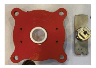
2.2.3 Place the new position indicator assembly (1 - 140) onto the yoke (1 - 70), make sure the spring pin (1 - 100) is in the slot of the position indicator assembly (1 - 140) plate.
