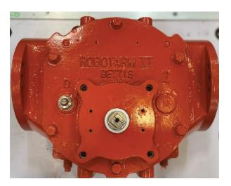
2.2.5 Install and tighten the new Hex head screws (1 - 160) and washers (1 - 170). Install new position indicator (1 - 220).
