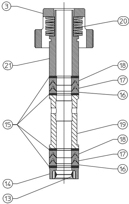
Figure 5. ENVIRO-SEAL Graphite ULF Packing Arrangement
