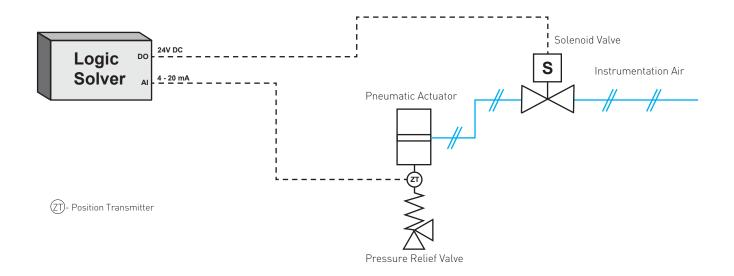
VALVE POSITIONER/DIGITAL VALVE CONTROLLER(2)[4][5]
