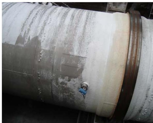
*Three 648 wireless temperature transmitters were installed with RTD's and thermowells and distributed along the length of the dryer, 120° out of phase.*
