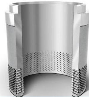
*The Cavitrol III cage has specifically shaped holes, spaced diametrically around the cage circumference. These holes reduce fluid turbulence, dissipate fluid pressure, and help increase flow capacity.*
