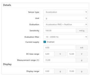
From picture above you can find a typical configuration example of the VI Piezo CHARM for a 2-wire piezoelectric ICP® Accelerometer Sensor being connected.
