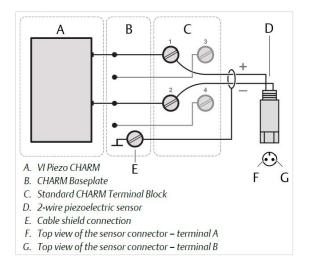
Apply the connections to the 2-wire piezoelectric ICP® Velocity Sensor as shown above and make sure the current supply is either provided by the VI Piezo CHARM. directly or externally (where required).
