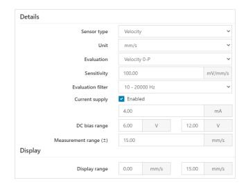
From the picture above you can find a typical configuration example of the VI Piezo CHARM for a 2-wire piezoelectric ICP® Accelerometer Sensor being connected.
