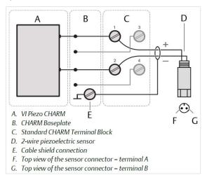
Apply the connections to the 2-wire piezoelectric ICP® Accelerometer Sensor as shown above and make sure the current supply is either provided by the VI Piezo CHARM directly or externally (where required).
