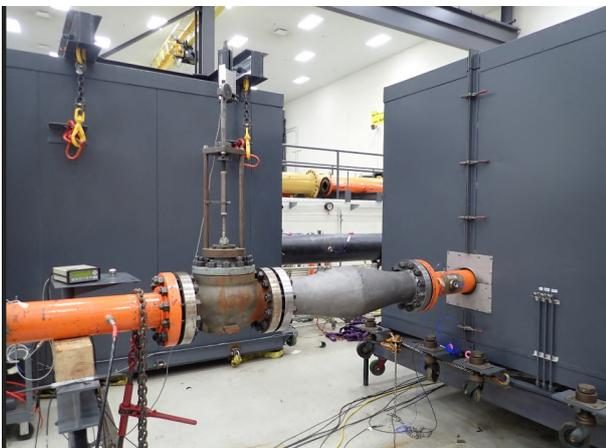
**Figure 3.** The forged WhisperTube (6 in. model shown) undergoing noise testing at the Emerson Innovation Center Flow Laboratory.
