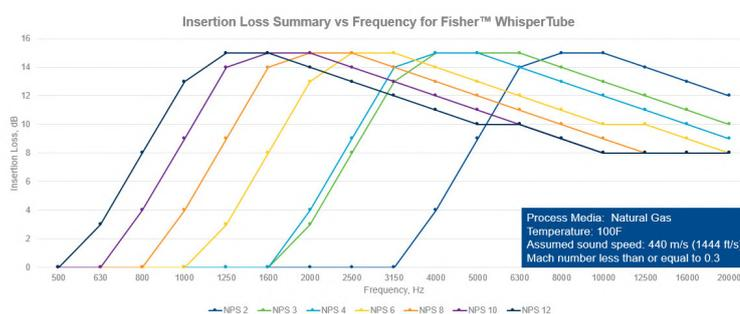
**Figure 5.** Concentric rings of various sizes create broadband noise reduction as shown in this chart. Generated noise and rejected frequencies tend to shift higher as pipe size is reduced, so the suppressor is well matched to the typical application.
