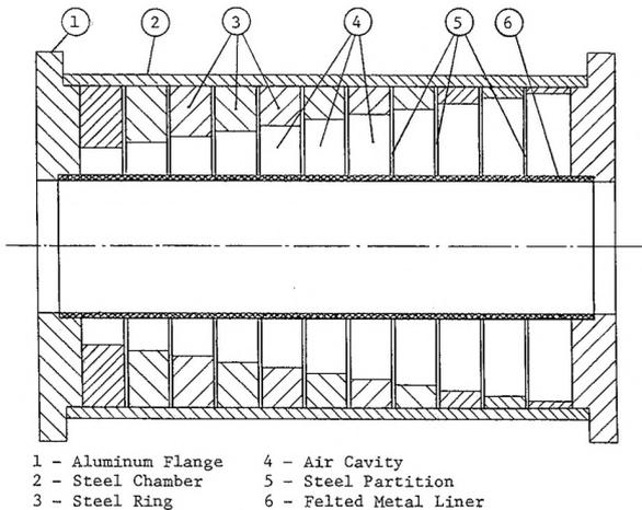
**Figure 2.** This diagram shows the original concept of a modal coincidence suppression device, designed to reduce the aerodynamic noise produced by a control valve. The series of chambers are each sized to produce destructive interference across a small range of frequencies.
