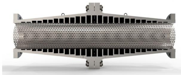
**Figure 4.** The modal suppressor consists of cylindrical chambers of varying sizes surrounding a full bore perforated tube. Each chamber generates destructive interference over a small range of frequencies to provide significant noise reduction across a broad spectrum.
