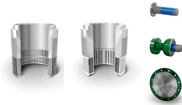
**Figure 1.** Source control often uses valve trims with small holes (left), multiple flow paths (middle), or downstream diffusers (right) to reduce aerodynamic noise. The methods spread the pressure drop and flow across multiple points to reduce vapour velocity and minimise noise.
