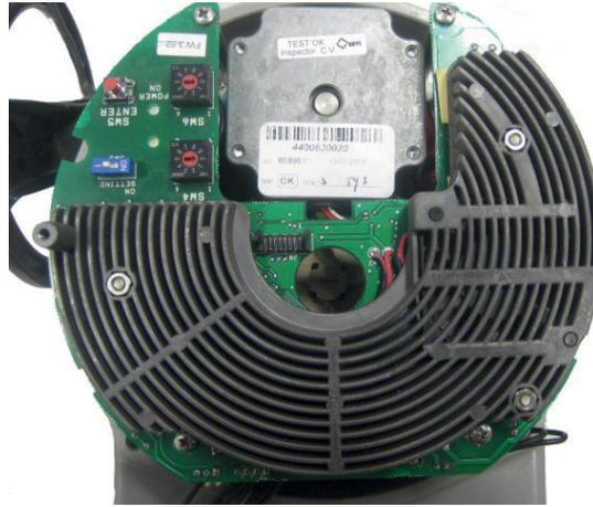
**Figure 4** Example of EPI2 new version (heatsink not present)
