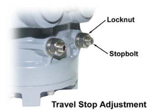
**☞** Do not set the Actuator position limit switches to drive into the mechanical stops. Damage can occur of electric unit is allowed to repeatedly stall into the end stops.
