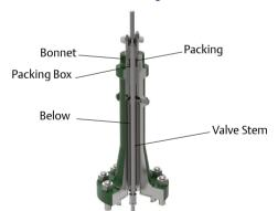
ENVIRO-SEAL bellows seal bonnets improve sealing capabilities of Fisher valves and provide long life for applications where emissions escaping from a valve stem seal to the atmosphere cannot be tolerated. This excellent stem sealing system is available for Fisher easy-e and Fisher GX valves.
